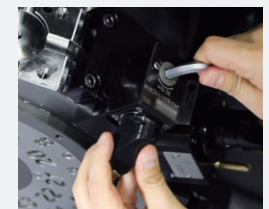
Quick change tooling (CAPTO)
