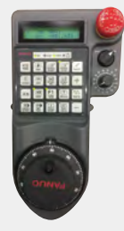
Manual operation panel
